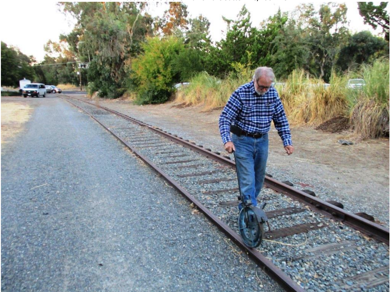
Then measures the length of the track between Sutterville Road and South Land Park Drive. There is room for a run around track.
