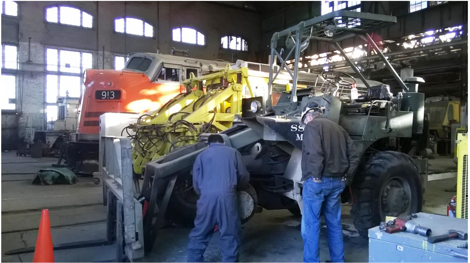
Alan supervises the mechanic from Valley Forklift who is working on replacing Big Green Machine's brake calipers
