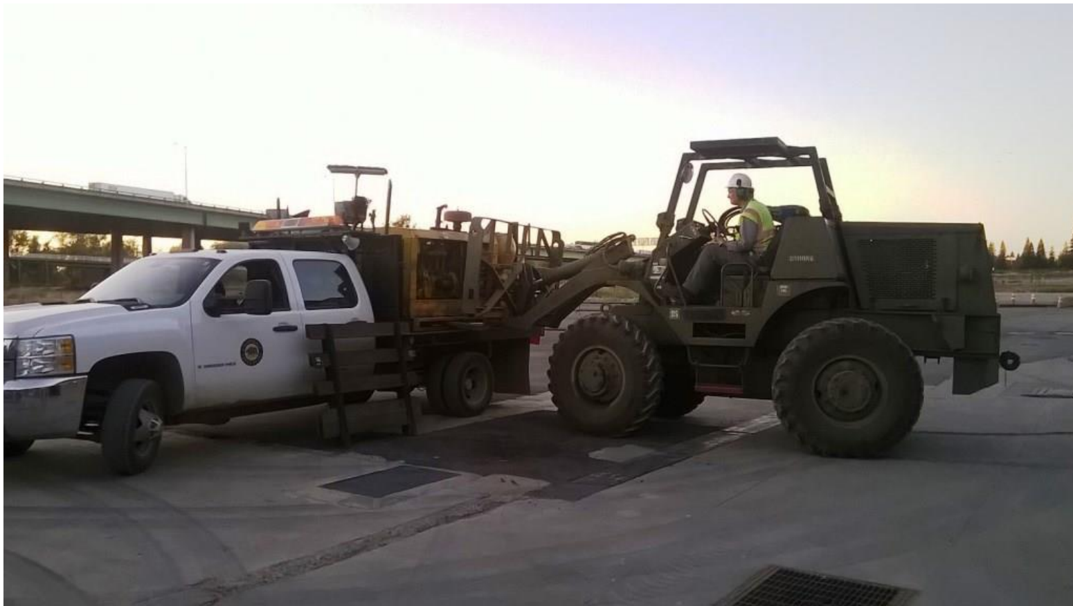
With GM2's brakes certified as 100% efficient, Steve removes the rail-mounted air-compressor's engine from the truck
