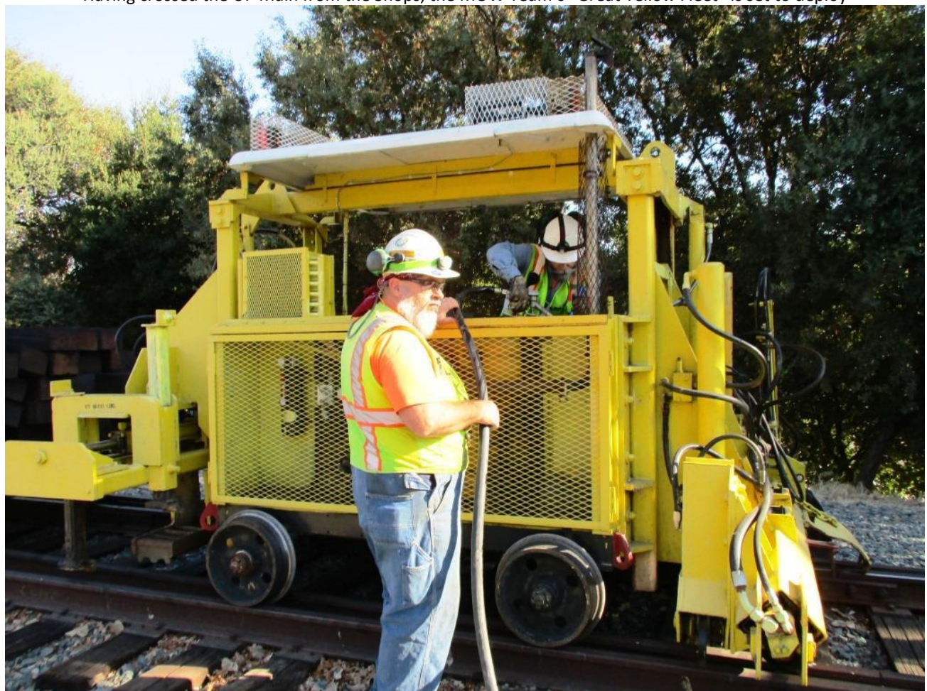
At Baths, Mike F. and Joe feed fresh diesel to the Jackson 125 tie-exchanger
