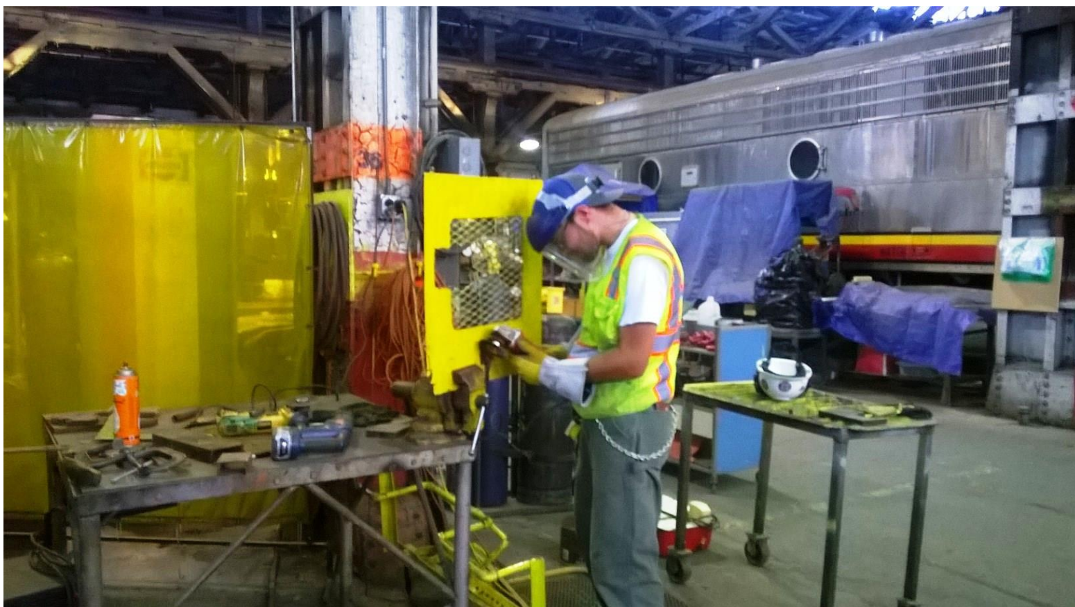
Kyle makes the final modifications to the Kalamazoo's engine cover to fit its new air-compressor
