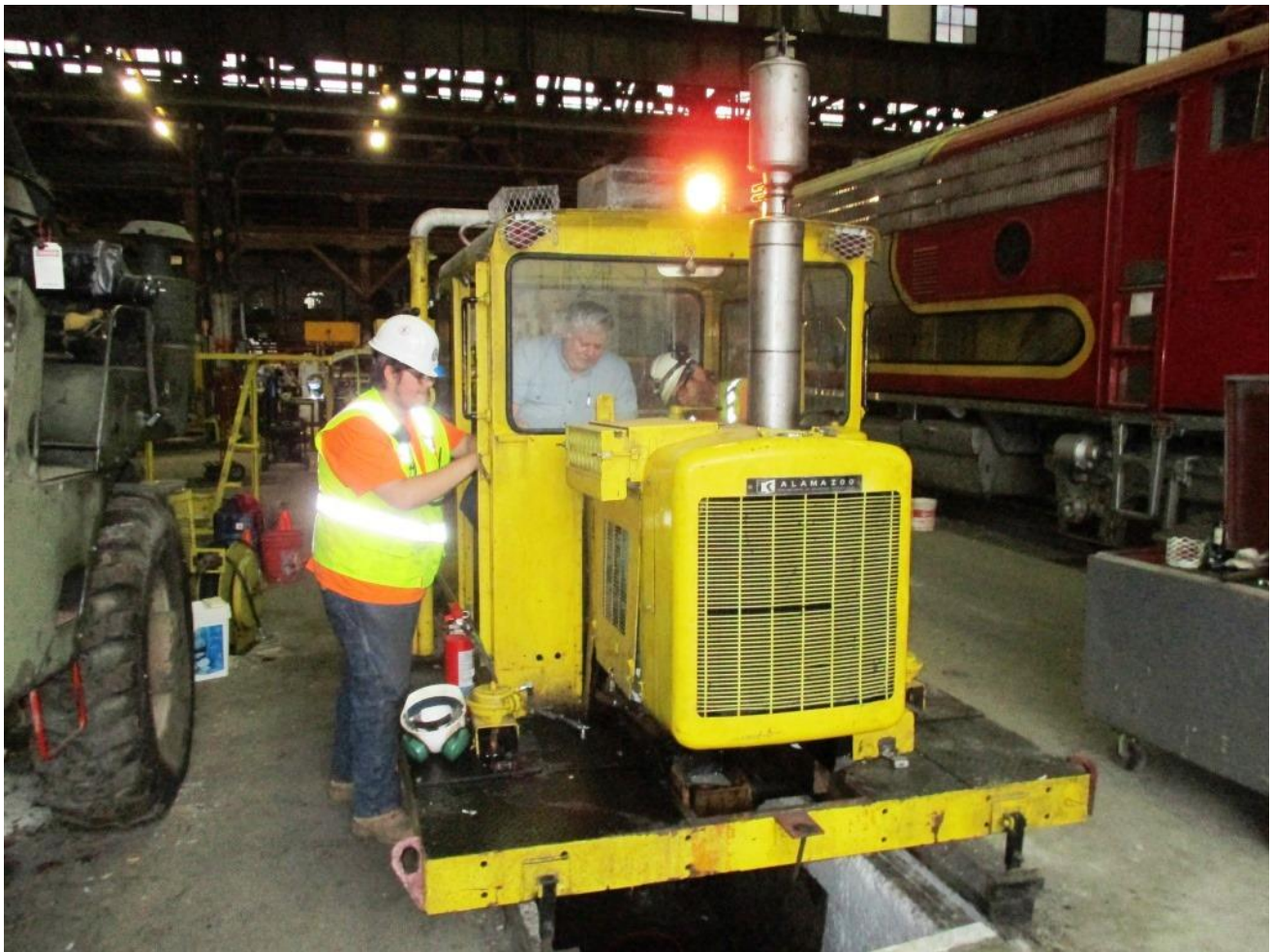
Chris H., Chris C., and Joe fire-up the Kalamazoo and get it ready to roll under its own power for the first time with its new engine
